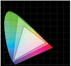
The colour gamut of a LED based projector is much greater than that of a traditional lamp based projector, resulting in deep, saturated colours.
