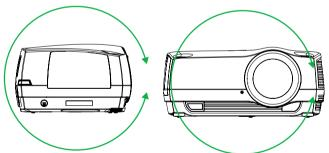
The FL32 can be rotated 360 degrees around around all axes without any loss of performance.
