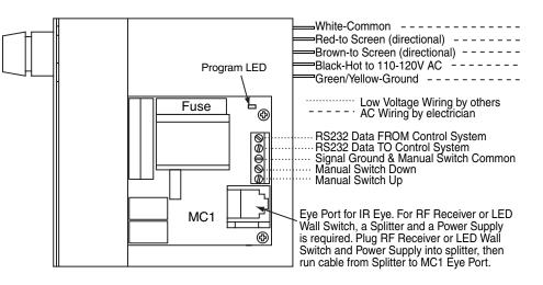
See separate Serial Communication-RS232 Instruction sheet for enabling RS232 with the MC1.
