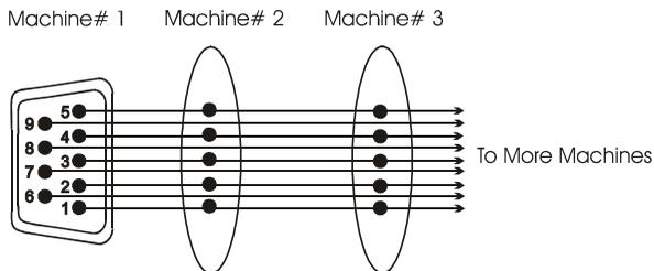
Figure 3: Connecting Multi-Machines
