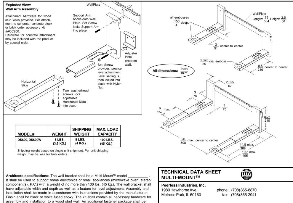
available to enable installation to solid concrete and concrete block walls.
