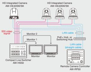
\*The AC adaptor provided with the unit is not shown in the above figure.
