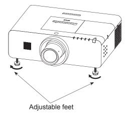
Adjustable range Front adjustable feet : 30 mm (1.181")
