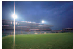
Conventional CCD Sensor (vertical smear)
