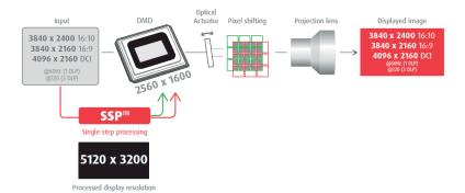
Figure 2. The 4K UHD method in a Barco projector
