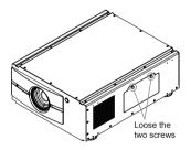
3. Use a screw driver to loosen the screws as shwon in the illustration.
