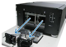
5. Insert the new lamp in the direction shown in the illustration into the lamp assembly; tighten the two screws using a screw driver and make sure the lamp is firmly secured to prevent the lamp from shaking or poor contact.
