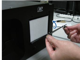
3. Reattach the filter cover and tighten the two screws.
