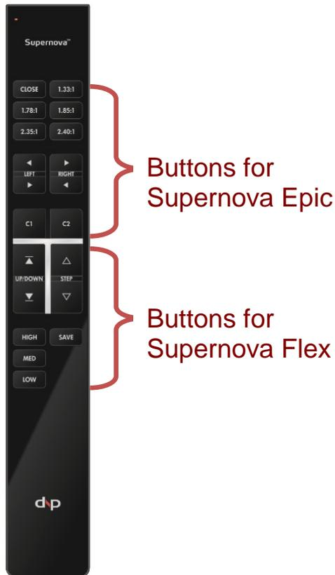
**NOTE!** Be aware when installing the screen close to equipment using the same IR communication protocol. Commands may activate other electronic components. (see installation manual for details).
