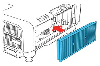
5. Attach the air filter cover as shown, and press it gently until it clicks into place.
