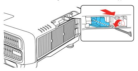
4. Insert the wireless LAN module into the port.
