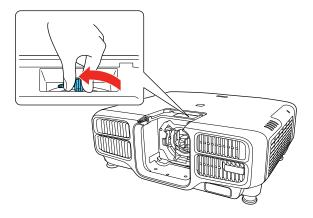
4. Insert the lens straight into the projector's lens socket with the white dot facing up.
