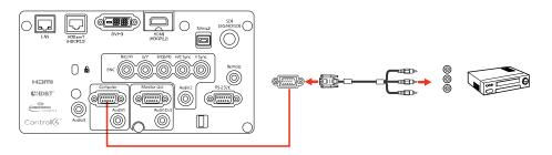
3. Tighten the screws on the VGA connector.
