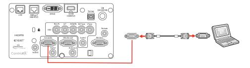
4. Tighten the screws on the VGA connector.
