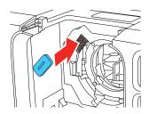
3. Slide the lock lever to the **Release** position (as shown) until you hear it click.
