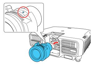
5. Hold the lens firmly and slide the lock lever to the **Lock** position (as shown) until it locks.
