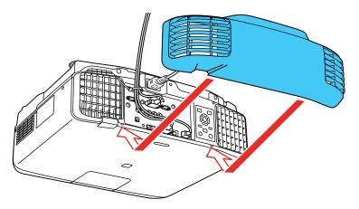
3. Tighten both cable cover screws.
