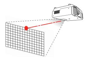
**Note:** If you installed the optional ELPLU02 short throw lens and you see a message prompting you to manually adjust the image distortion, manually rotate the distortion ring counterclockwise. Adjust the focus and then rotate the distortion ring again to correct image distortion.
