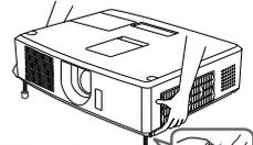
To loosen an elevator foot, push the elevator button on the same side as it.
