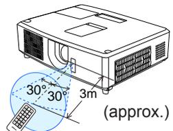
**NOTE** • You may be able to reflect the remote control signal from the screen. If you are having difficulty sending the signal to the sensor directly, try reflecting the signal.
