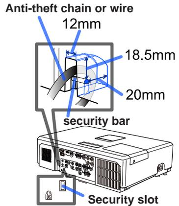
**⚠ WARNING** ▶ Do not use the security bar and slot to prevent the projector from falling down, since it was not designed for this purpose.
