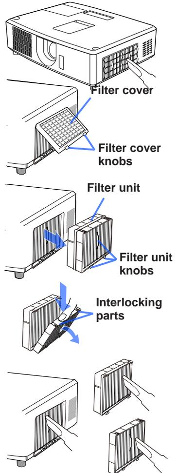
**Cleaning and replacing the air filter (continued)**
