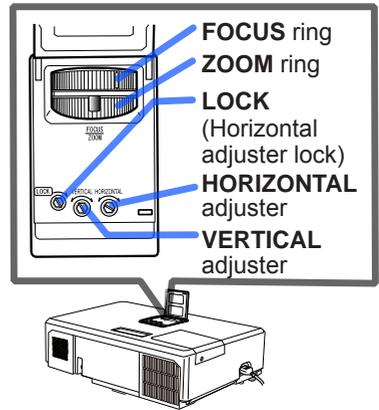
**⚠ CAUTION** ▶ Operate the lens adjustment controls gently as the lens may malfunction when subjected to jolts. You may need to use more strength using the controls near the end of their range. Be careful not to apply too much strength.
