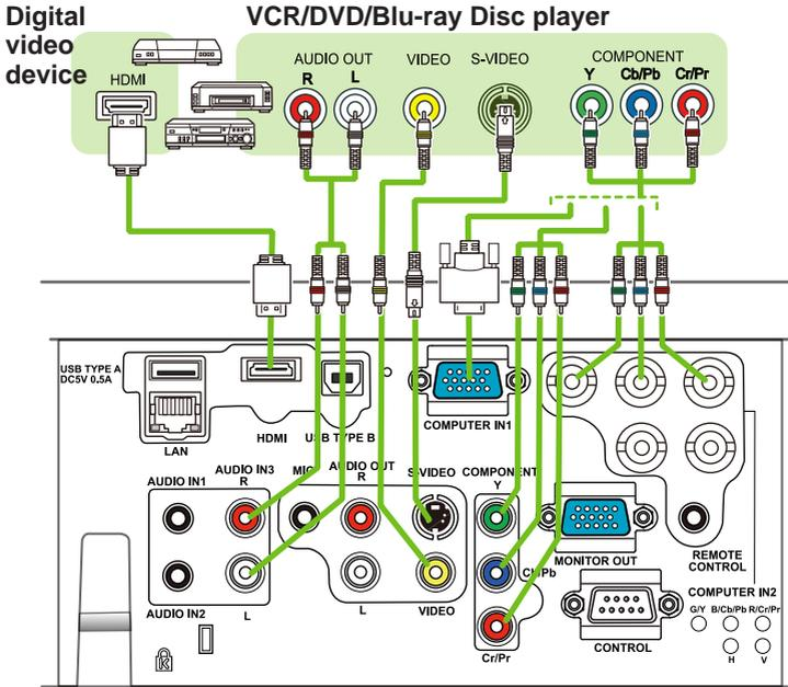
**NOTE** • The **HDMI** port of this model is compatible with HDCP (High-bandwidth Digital Content Protection) and therefore capable of displaying a video signal from HDCP compatible DVD players and the like.
