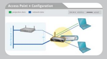
Let LiteShow II function as a wireless network access point. Simultaneously transmit presentation material and access the network and Internet. Improve network access and enable wireless presentation – all from the same device.
