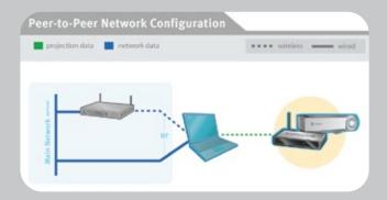
No network setup necessary; all software is hosted on LiteShow II. Communicate directly from your PCs wireless card to the LiteShow II adapter. No network connectivity in this mode makes it ideal for guest presenters.
