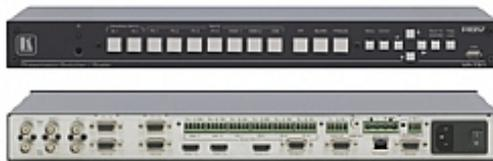
The **VP-731** is a 9-input scaler/switcher for analog video, digital video, balanced stereo and S/PDIF audio signals. It up or down-scales composite, s-Video (Y/C), component video (YUV), HDMI, computer graphics video and JPEG files to a selectable computer graphics video or HDTV output resolution on one HDMI and two 15-pin HD outputs. The **VP-731** is the same as the VP-730 with the addition of Ethernet control.
