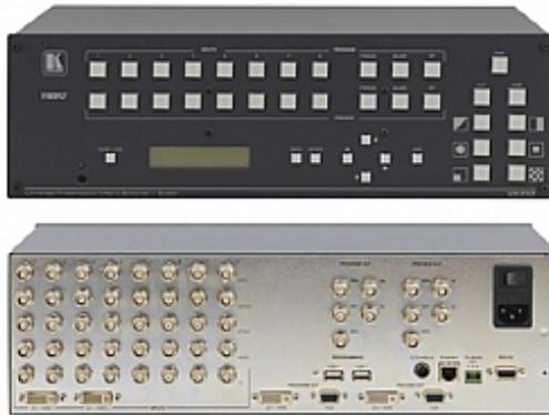
The **VP-747** In-CTRL Dual Scaler Seamless Switcher is a true multi-standard scaler and seamless switcher with 8 universal inputs comprised of 5 BNCs each, any of which can accommodate a composite video, s-Video (Y/C), component video (RGB/YUV), RGBS, or RGBHV signal. Inputs 1 and 2 also can be configured to HDMI/DVI inputs. The unit has dual scalers, one for the preview and the other for the program output. Dual scalers are required to do “true” seamless transitions from one source to another.
