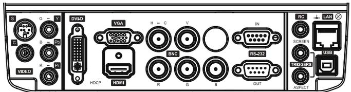
The comprehensive input panel features two digital video inputs, in addition to comprehensive control and command interfaces, compatible with for instance AMX and Crestron home automation systems.
