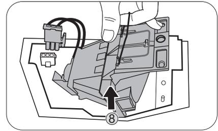
9. As shown in the figure, insert the new lamp. Align the lamp connector and 2 sharp points with the projector and push the lamp a bit into the locked position.
