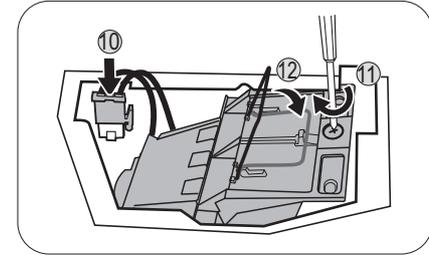
11. Tighten the screw that secures the lamp.
