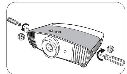
15. Tighten the screws that secure the lamp cover.
