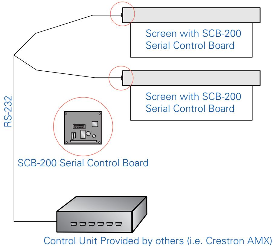
The SCB-200 screen controller provides control over a screen using RS-232C communications or an optional Ethernet controller, wall controller or infrared controller. Designed for applications where precise screen control and monitoring capabilities are crucial, the SCB-200 is available as a factory installed option in the Contour, Tensioned Contour, Advantage, Tensioned Advantage, Advantage Deluxe, Tensioned Advantage Deluxe, Director and Tensioned Director Electrols.
