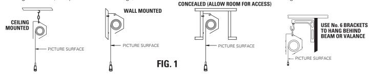
**NOTE:** Under no circumstances should unit be completely sealed in recessed installation. Allow access for service. Picture surface is centered in case. Case extends 5-1/2" beyond surface on either end. Do not attach anything to screen slat rod or bottom fabric pocket.
