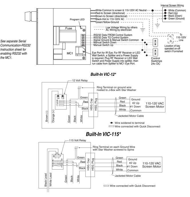
\*These wiring diagrams are for Access screens with motor on audience left (standard), and fabric unrolling from the back of the roller (standard).
