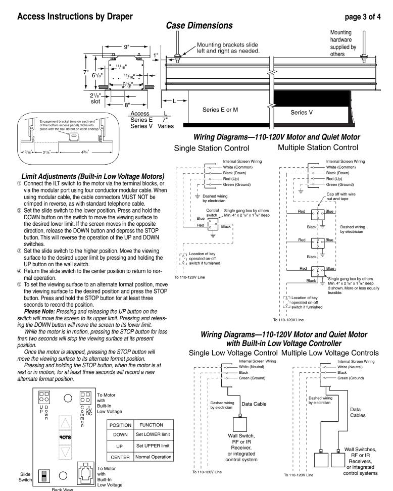
\*These wiring diagrams are for Access screens with motor on audience left (standard), and fabric unrolling from the back of the roller (standard).
