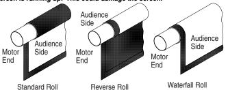
Standard/Reverse Roll Left hand motor White Socket—Down Yellow Socket—Up Right hand motor White Socket—Up Yellow Socket—Down
