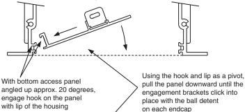
Engagement bracket (one on each end of the bottom access panel)
