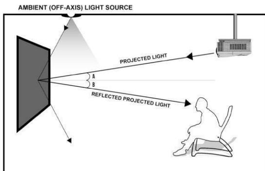
**Projector Table Top:** Make sure the projector (*light in*) is angled (A) to reflect (B) at the mirror-opposite angle (*light out*) to align with the viewer’s eye level.
