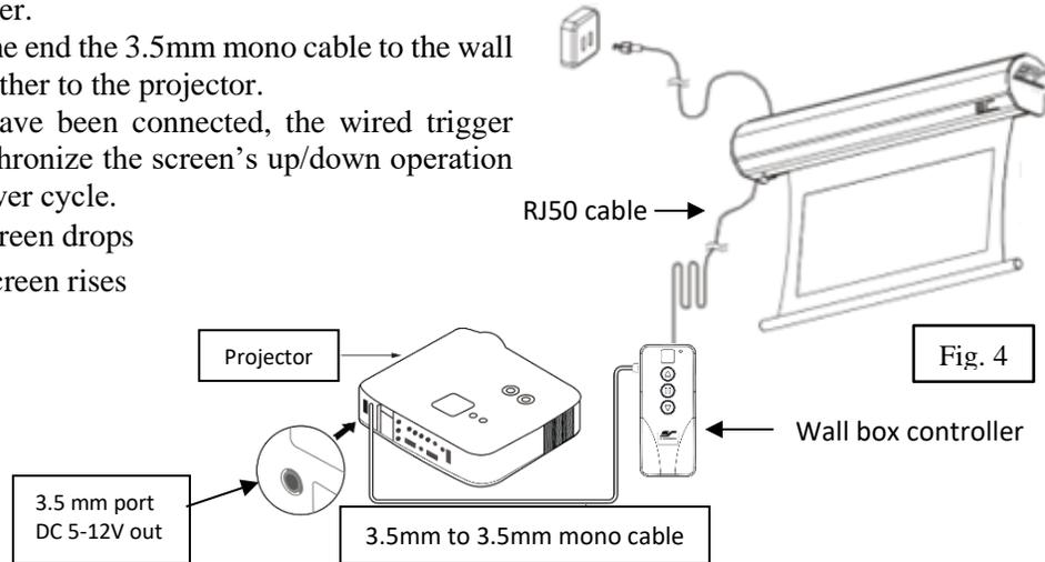
**5. Wireless 5-12 volt trigger (Fig 5):** Requires a 3.5mm to 3.5mm mono cable (not included).
