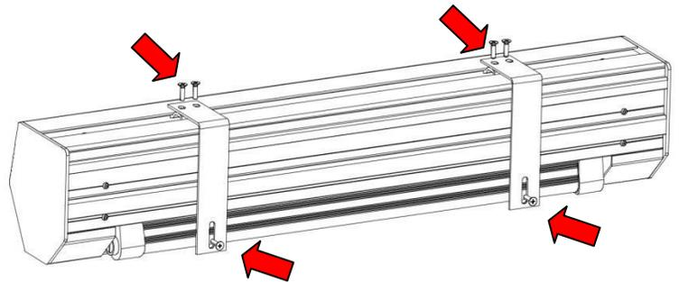
**NOTE:** Regardless of the mounting method, each screen should be securely installed so that vibrations or pulling on the viewing surface will not cause the casing to become loose or fall. Included are complimentary mounting screws that may or may not be appropriate for your installation. Always use the correct anchors to safely secure the screen and always consult a professional integrator.
