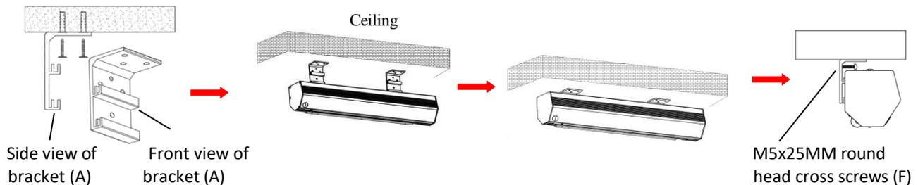
1. Determine where the screen will be installed. Then, measure and mark the distance between the top and bottom screw holes from each **Wall/Ceiling mount bracket (A)**.
