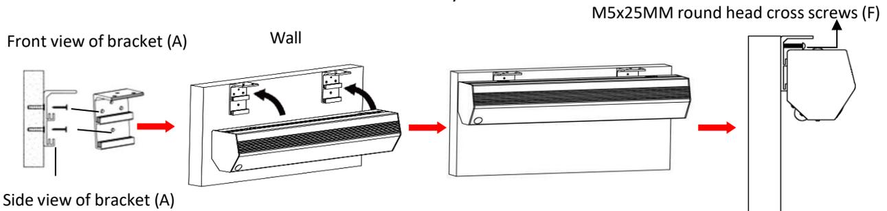
1. Determine where the screen will be installed. Then, measure and mark the distance between the top and bottom screw holes from each **Wall/Ceiling mount bracket (A)**.
