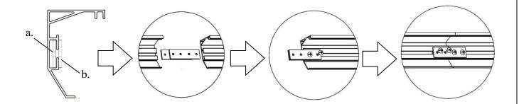
**Step 4:** Connect the *elbow joints* (*c/d*) to the top and bottom sections of the vertical frame. Once inserted, connect the vertical sections to the horizontal frame sections. Make sure all holes are in alignment and the frame pieces are flush (no gaps). They should form perfect right angles.
