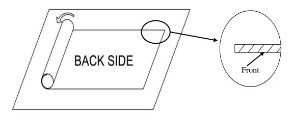
**Step7**: Carefully place the screen on top of the assembled frame as shown below. Make sure that the angular **edges** of the frame are not allowed to come into direct contact with the screen material to avoid puncturing.
