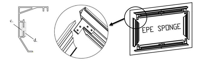
**Step 5.** Secure the elbow joints by fastening them with M4x7 screws (g), 4 at each corner.
