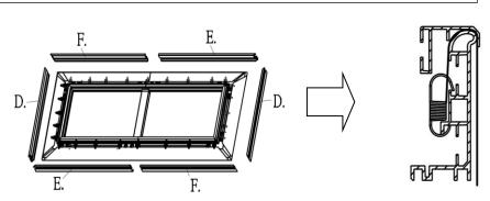
Connect edge trim frames (e/f) together using the Center Joints- M4(a) and secure with four of the M4x4 Screws (m) as shown in Step 1. Repeat for other side.
