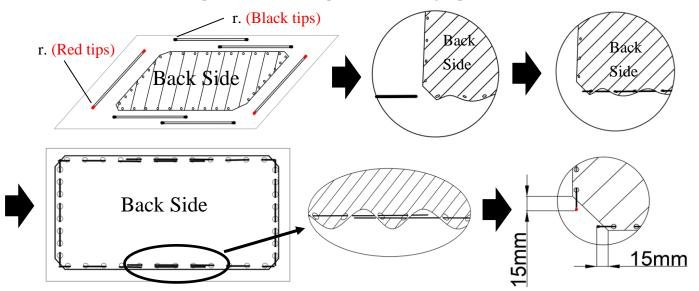
**Step 8:** Carefully and gently place the assembled frame on top of the screen material in the marked areas as shown below. Make sure to not allow the angle edge of the frame to come in direct contact with the screen material to
