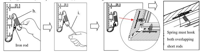
Begin by first attaching the center points on both vertical (left/right) sides, *steps 1-2*. Then the center points on both horizontal (top/bottom) sides, *steps 3-4*. Once all center points have been secured, make sure the screen material is still within the marked areas before proceeding to attach the next springs.
