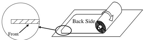
**Step 7:** Insert the rods(r) through the holes according to their corresponding lengths on each edge of the screen material as shown below. The short rods (top/bottom) will overlap to secure a firm grasp in the middle areas.
