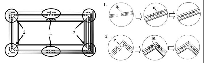
**Step 12**: Install the *angle cover* (n) on each corner of the frame as shown in the illustration below.
