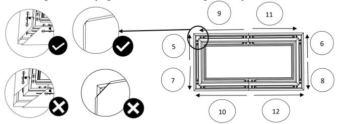
To avoid ripples forming in the material it is imperative that all of the corners are properly wrapped around the edges as illustrated in the check mark diagrams.
