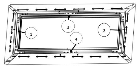
Continue attaching the rest of the springs to the material in the following order in *steps 5-12*.
