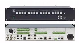
The VP-23N is a 4x1 composite video, a 4x1 s-Video (Y/C) and 4x1 computer graphics video switcher, each with balanced stereo audio. It is designed for a wide variety of presentation and multimedia applications.
