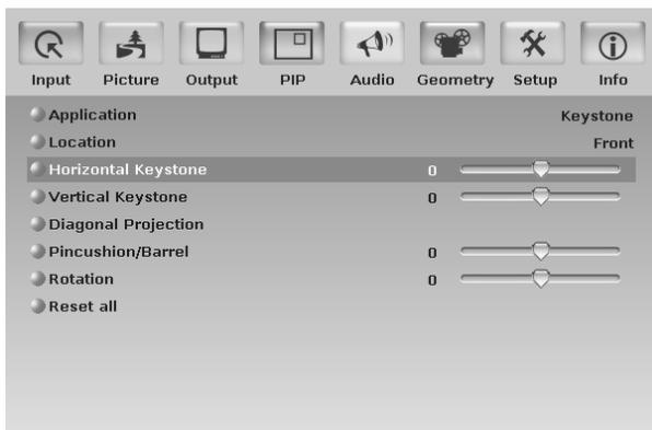
Figure 14: Geometry Screen
