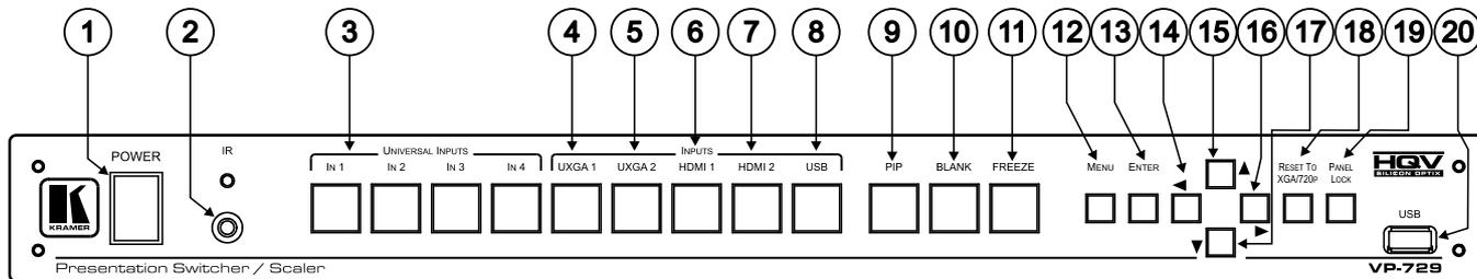
Figure 1: VP-729 Presentation Switcher / Scaler Front Panel
