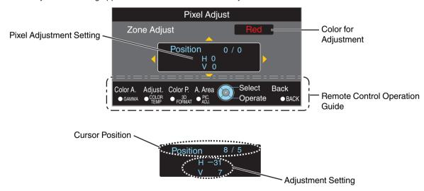
① After adjustment is complete, press the [BACK] button twice to exit the Adjustment mode
