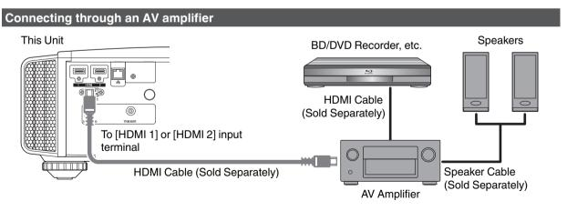
If the source device is connected to the projector through an intermediate device such as an AV amplifier or divider, the video image may not appear depending on the specifications of the intermediate device.
