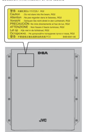
As with any bright light source, do not stare into the beam, RG2 IEC 62471-5:2015
