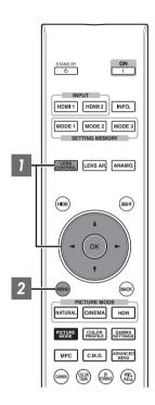
Press the [LENS CONTROL] button, and use the [AV > ] keys to adjust Focus, Zoom (screen size), and Shift (screen position)
