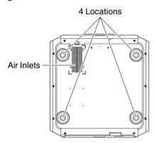
Remove the four feet at the bottom, and fasten using the screws (M5 screws, 13 to 23 mm).
