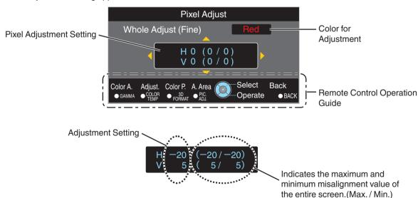
(f) After adjustment is complete, press the [BACK] button twice to exit the Adjustment mode
