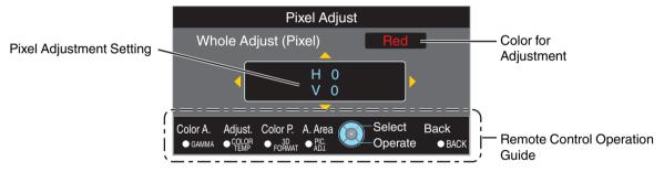
(f) After adjustment is complete, press the [BACK] button twice to exit the Adjustment mode
