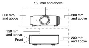
Leave the front area of the unit unblocked. If there is any obstructing object in front of the exhaust vent, hot air will flow back to the unit and cause it to heat up. Hot air flowing out of the unit may cast shadows on the screen (heat haze phenomenon).
