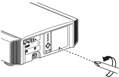
**3** Loosen the screws of the lamp unit
