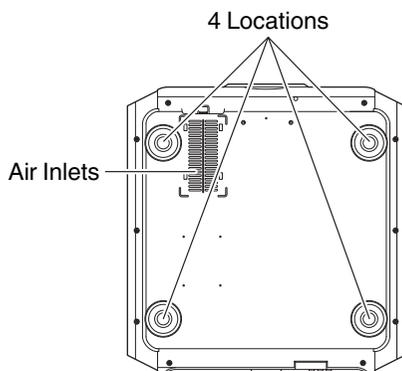
Remove the four feet at the bottom, and fasten using the screws (M5 screws, 13 to 23 mm).
