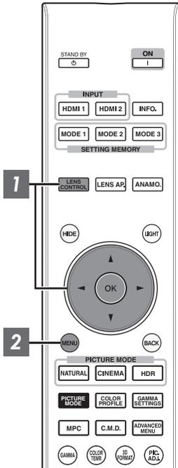
**1** Press the [LENS CONTROL] button, and use the [▲▼◀▶] keys to adjust Focus, Zoom (screen size), and Shift (screen position)
