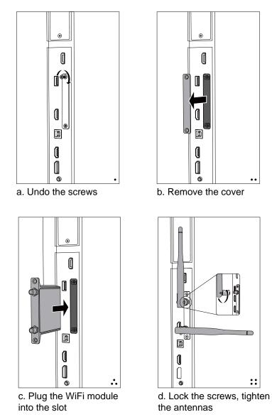
Note: This wifi module only works for the IFP by plugging it into the above slot.
