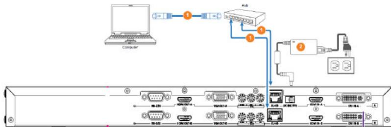
To connect the blending box with other devices, there should be cables listed as below
