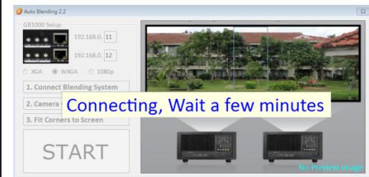
3. Ensure input/output timing setting is the same between GB1000 & Projector. Re-click if you see magenta flashing screen in 10 seconds.
