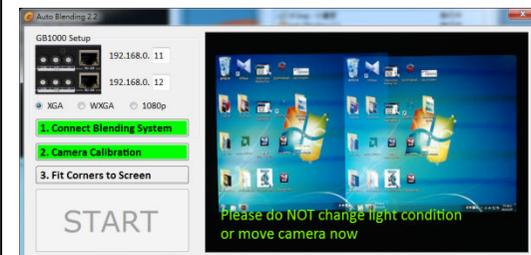
6. Click "Fit to Screen" to adjust L/R projector display four corners. Each marker movement can be adjusted by changing pixel range (1~7 pixels of each movement).
