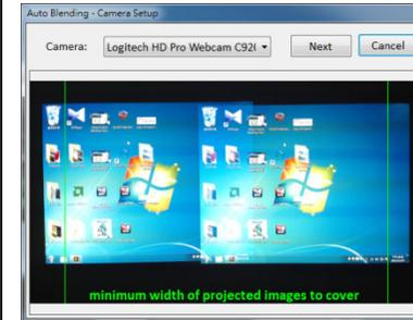
5. Click "Camera Calibration" to optimize camera. Do not change environment lighting condition once calibration completed.
