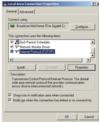
6. Fill in the IP address and Subnet mask, then press **OK**.
