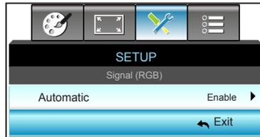
Automatically selects the signal. If you use this function, the Phase, frequency items are grayed out, and if Signal is not automatic, the phase, frequency items will appear for user to manually tune and saved in settings after that for next time projector turns off and on again
