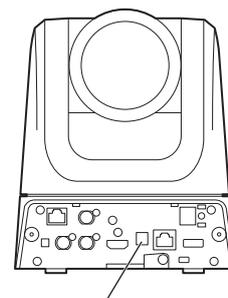
Wireless remote control signal light-sensing area
