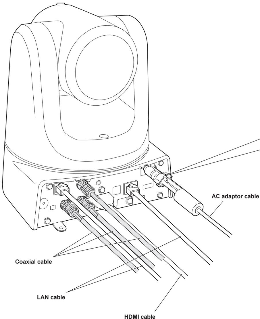
● How to secure the AC adaptor cable
