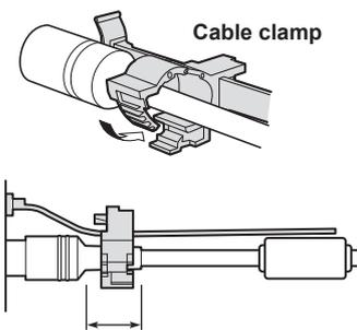
Loosely secure the cable clamp in the area shown above.
