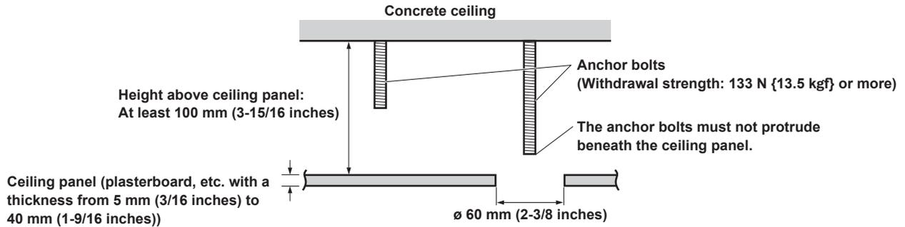
1. Refer to the Operating Instructions of the WV-Q105A direct ceiling mount bracket, and attach the WV-Q105A as well as the drop-prevention wire angle and drop-prevention wire supplied with the WV-Q105A to the anchor bolts.
