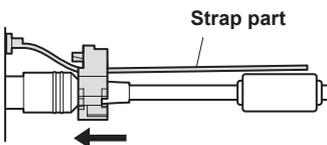
Take hold of the strap part, slide the cable clamp until it stops moving, and then secure it tightly.
