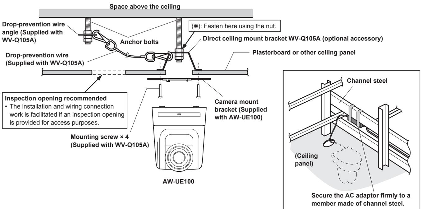
3. Install the AW-UE100 camera by following the procedure starting with step 3 on page 9.
