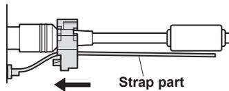
Take hold of the strap part, slide the cable clamp until it stops moving, and then secure it tightly.
