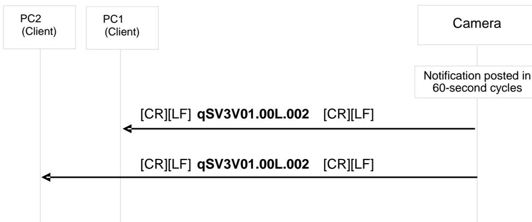
Fig.4-8 Sequence when the version information is received
