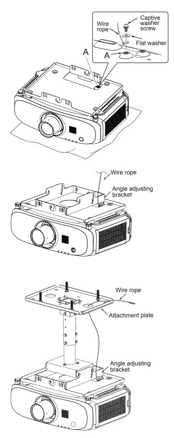
1 Secure one end of the wire rope with a captive washer screw (M6×20) to "A" on the projector as shown on the left.
