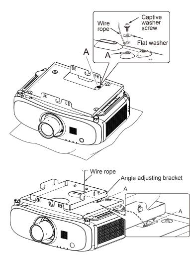
1 Secure one end of the wire rope with a captive washer screw (M6×20) to "A" on the projector as shown on the left.
