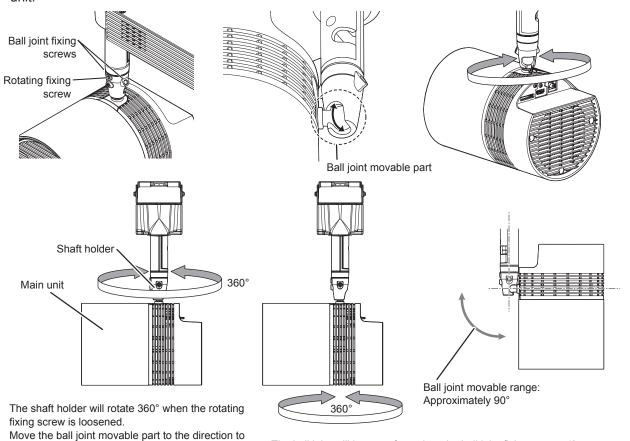
The ball joint will become free when the ball joint fixing screws (2 locations) are loosened.
