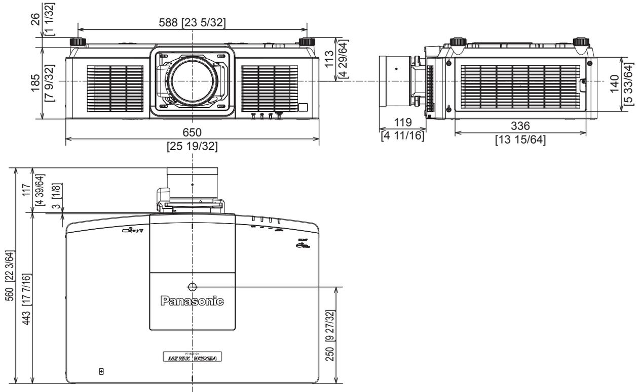
\* The above dimensions are obtained when the standard zoom lens is attached.
