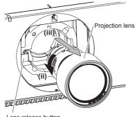
2) While pressing the lens release button, turn the projection lens counterclockwise to the end and remove.
