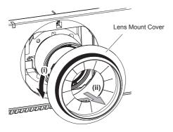
1) Turn the Lens Mount Cover counterclockwise and remove.
