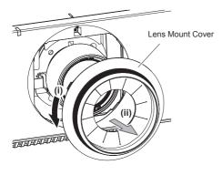
Remove the Lens Mount Cover, and align the projection lens guide to the guide groove of the projector and insert to the end.
