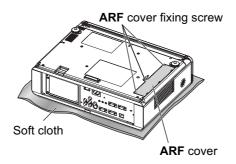
3. Use a Phillips-head screwdriver to loosen an ARF fixing screws and release the clamp, then slightly slide up the used ARF to remove.
