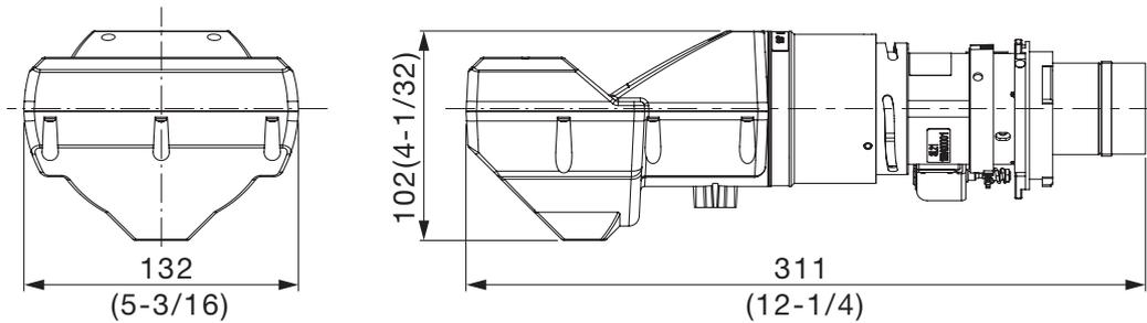
Illustration shows the lens attached to an applicable projector.
