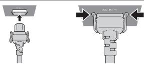
1) Check the shapes of the <AC IN> terminal at the rear of the projector and the power cord connector, and insert the connector completely in the correct direction (until you hear the side tabs click in place).
