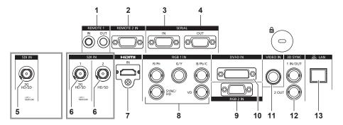
1 <REMOTE 1 IN> terminal/<REMOTE 1 OUT> terminal These are the terminals to connect the remote control for serial control when the system uses multiple projectors.
