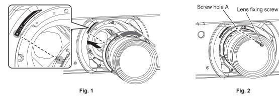
1) Insert by aligning the projection lens mark (orange) with the mark on the projector body (○ to the left of LOCK) and turn clockwise until it clicks. (Fig. 1)
