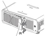
Lamp unit cover fixing screw
