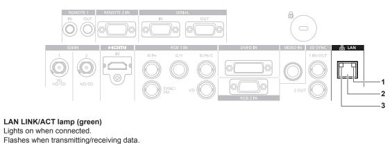
2 <LAN> terminal (10Base-T/100Base-TX) Used to connect the LAN cable here.
