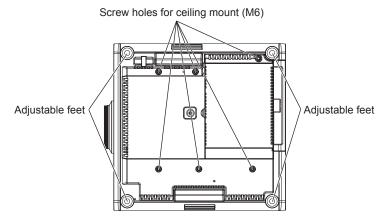
The positions of screw holes for ceiling mount and adjustable feet
