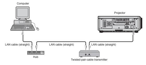
• For the LAN cable between a twisted-pair-cable transmitter and the projector, use a cable that meets the following criteria:
