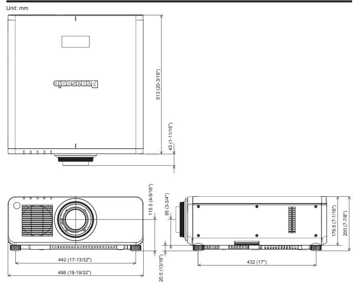
\* The above dimensions are obtained when the standard zoom lens is attached.
