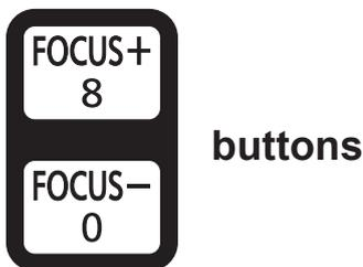
Press <FOCUS +/-> buttons on the remote control.
