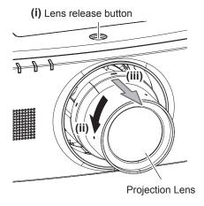
1) With the lens release button held down, turn the Projection Lens counterclockwise to the end and remove the Projection Lens.
