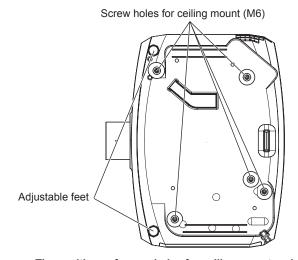
The positions of screw holes for ceiling mount and adjustable feet
