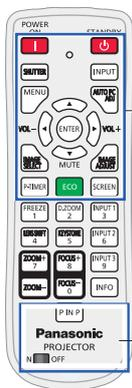
Only these buttons are active when the simple mode is set to [On]. [POWER ON, STANDBY, SHUTTER (AV MUTE), INPUT, MENU, AUTO PC ADJ., ▲, ▼ (MUTE), ◀ (VOLUME-), ▶ (VOLUME+), ENTER, IMAGE SELECT, IMAGE ADJUST, P-TIMER, ECO, SCREEN, P IN P, ON /OFF]. Number buttons also become active only when setting the remote control codes numbers or entering the PIN code numbers.
