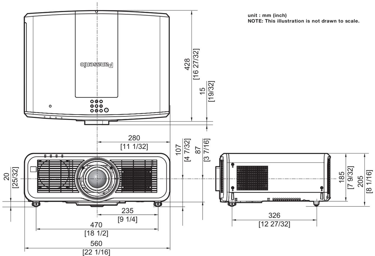
\* The above dimensions are obtained when the standard zoom lens is attached.
