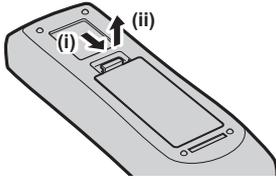
2. Remove the batteries.
