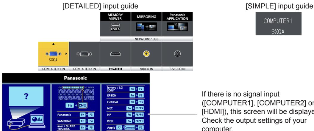
If there is no signal input ([COMPUTER1], [COMPUTER2] or [HDMI]), this screen will be displayed. Check the output settings of your computer.
