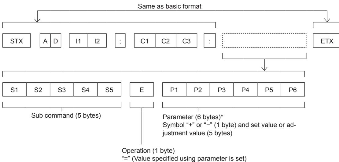
\* When transmitting a command which does not need a parameter, the operation (E) and parameter are not necessary.
