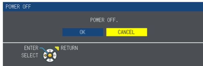
2) Press ◀▶ to select [OK], and press the <ENTER> button. (Or press the power <⏻/⏷> button on the control panel or the power standby <⏻> button on the remote control again.)
