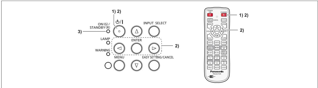
1) Press the power <⏻/⏷> button on the control panel or the power standby <⏻> button on the remote control.
